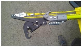
This tool is kept on T553. Notice the cutting edge is deep in the "jaw", the wire must be all the way in to successfully cut a drip loop.
